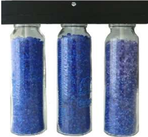
Assembled bottle array for silica gel
