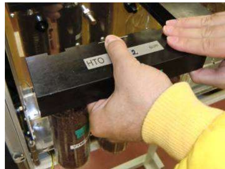
Insertion of the holder with sampling bottles with silica gel
