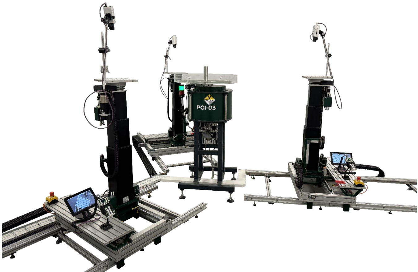
The PGI-03 irradiator equipped with a dosimeter rotating table and three CB-60 calibration benches
